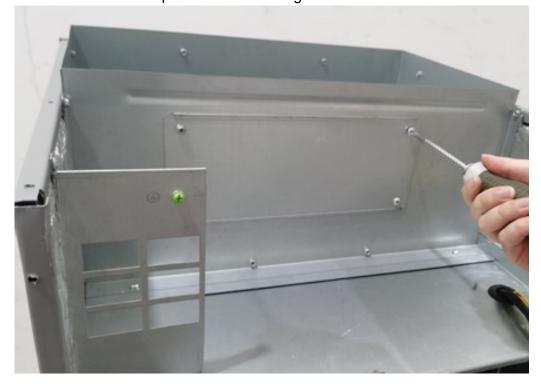
5. Install the electric heater to the metal plate position which disassembles in step 4. (Notes: There are two holes circled below which are used to fasten the electric heater bracket during installation)
