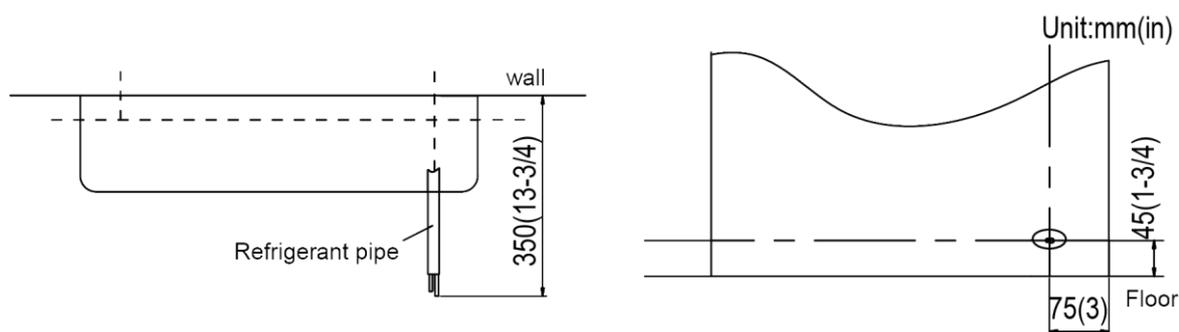
Boring a wall hole and installing wall embedded pipe.
